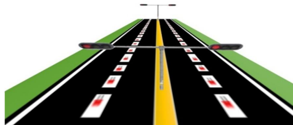
Fig .4 Arrangement of sensors in the middle of the roads.
