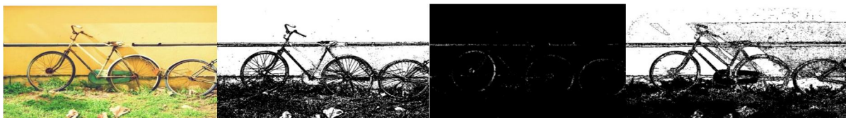
Fig. 2: (a) Sharp image with indistinct foreground and background (b) Y component (c) Cb component (d) Cr component
