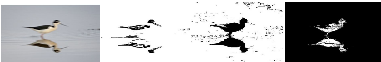
Fig. 2: (a) Blurred image (l = 25, a = 0) with semi distinct foreground and background (b) Y component (c) Cb component (d) Cr component
