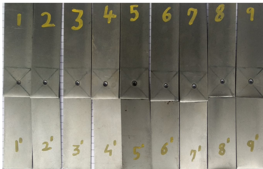
Figure 2.2 Resistance spot welding (RSW) Specimen.
