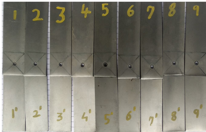
Figure 2.2 Resistance spot welding (RSW) Specimen.
