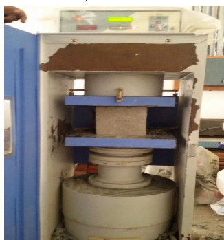
Fig. 2 Testing cubes for its compressive strength.
