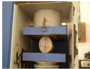
Fig. 3 Compression testing machine testing cylinders for tensile strength.
