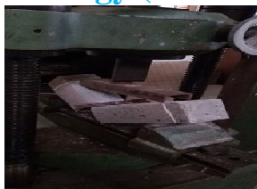
Fig. 4 Testing of beams for its flexural strength.
