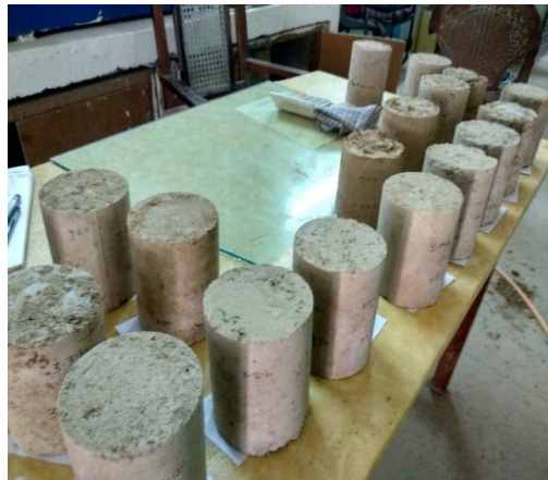
Figure 3 Wet-Dry Specimens after 7 day curing.
