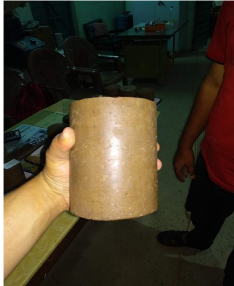
Figure 2. Specimen prepared for wet-dry test.
