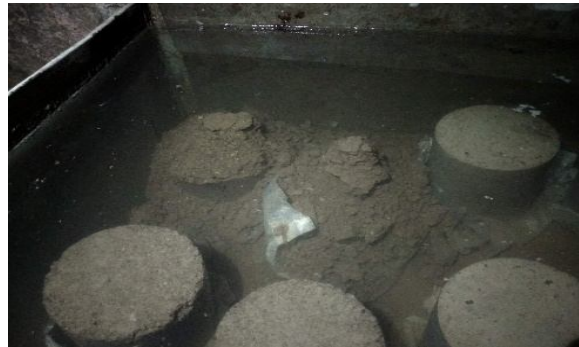
Figure 6 Breaking of specimen during wetting.
