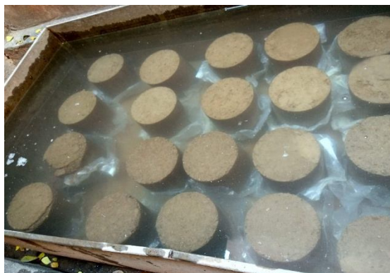
Figure 4 wetting phase of Wet-Dry test.
