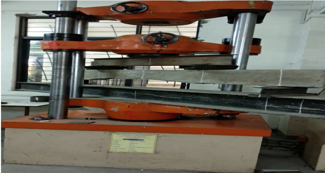
Photo 3 Two point loading set up
