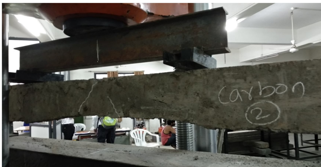
Photo 2 Testing of Haunched Beam
