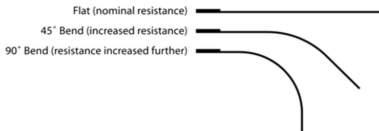
Fig.4 Flex Sensor Resistance Diagram
