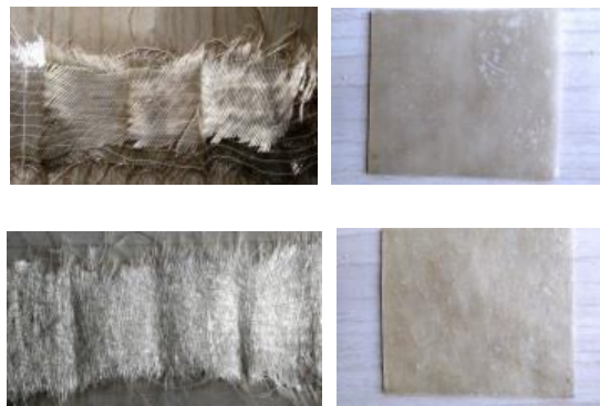
Fig.3. Glass mat and Glass Fibre Reinforced Polymer (GFRP)
