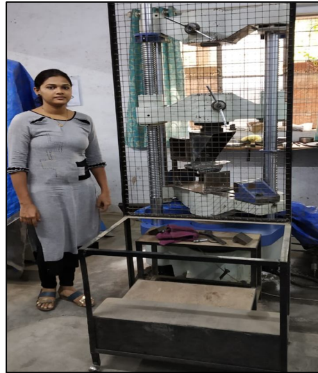
Fig.(6.4): Testing of Manufactured Bracket on UTM
