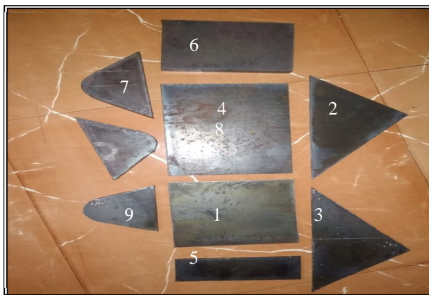
Fig. (6.2): Parts of super bracket shaped by laser cutting
