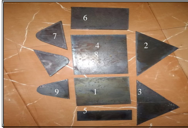
Fig. (6.2): Parts of super bracket shaped by laser cutting
