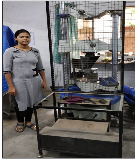
Fig.(6.4): Testing of Manufactured Bracket on UTM
