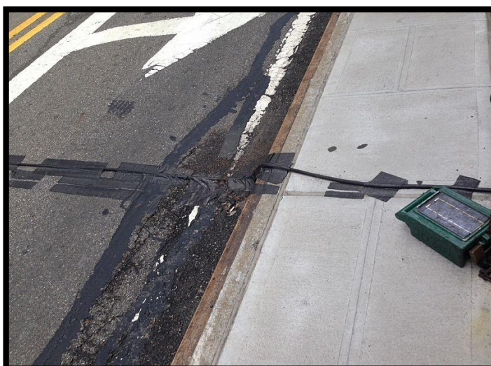
Fig. 2 Counter with tube on roadway and counting device on sidewalk
