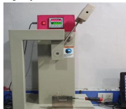
Fig.3. Izod impact test (ASTM D 256 - 2005)
