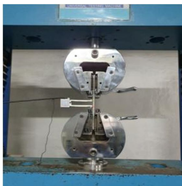
Fig. 2. Shear strength (ASTM D5379-12)
