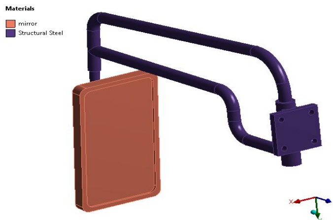
Fig no. 2 Existing RVSM material properties
