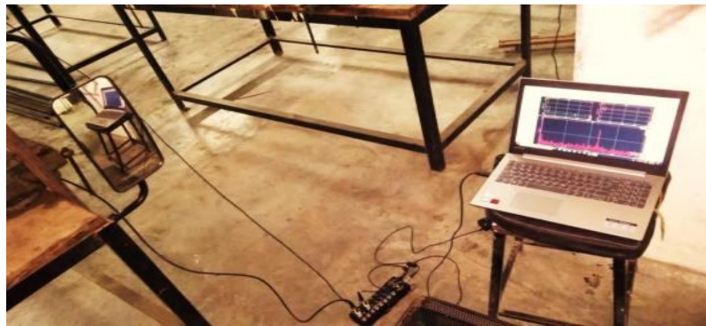
Fig no. 29 Experimental setup for Modal Analysis for Iteration 3 Design.
