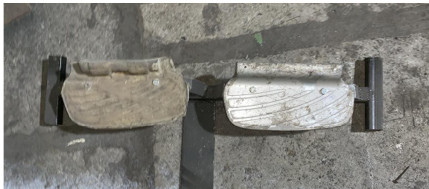
Fig.No.11 Actual Manufactured Model of Footrest
