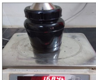
Fig. 3.2.1: Pycnometer filled with carbon black powder & water
