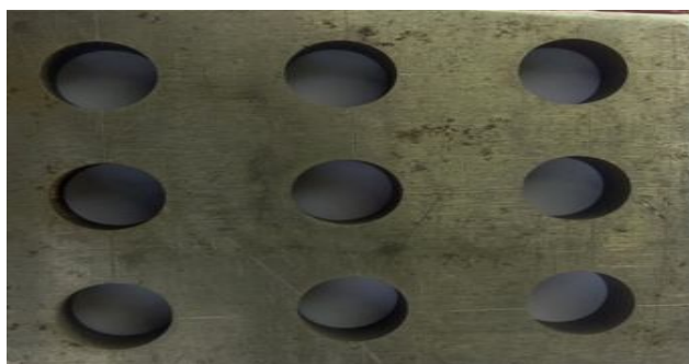
Fig. 2 After machining of holes on WEDM
