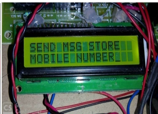
Fig. 4 LCD display of registering mobile number
