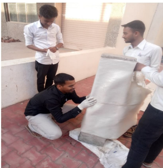
Fig.2. Wet lay-up system
