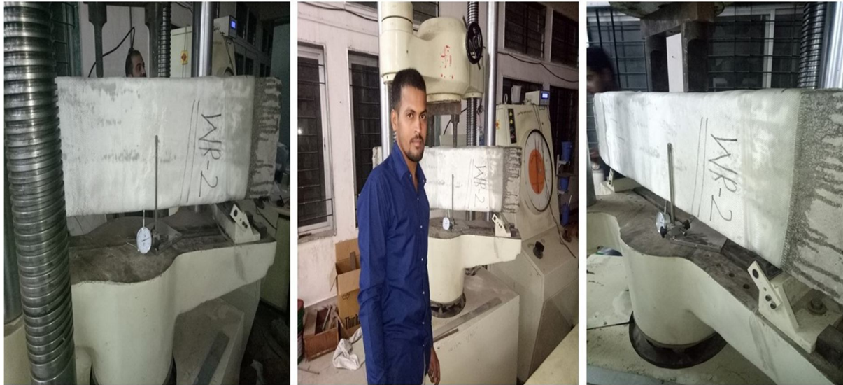
Fig.6. Testing of GFRP retrofitted RC beams
