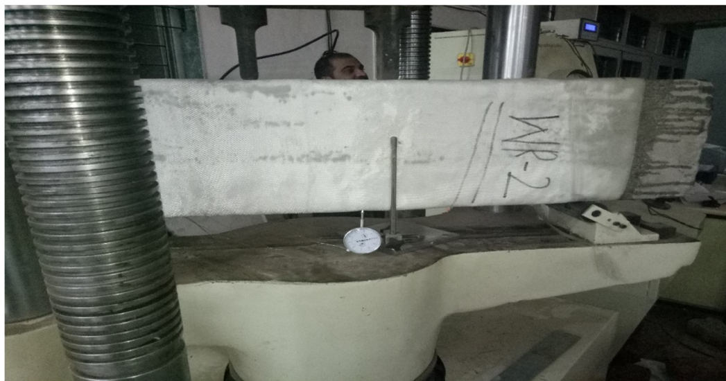
Fig.5. Experimental set-up of RC beams
