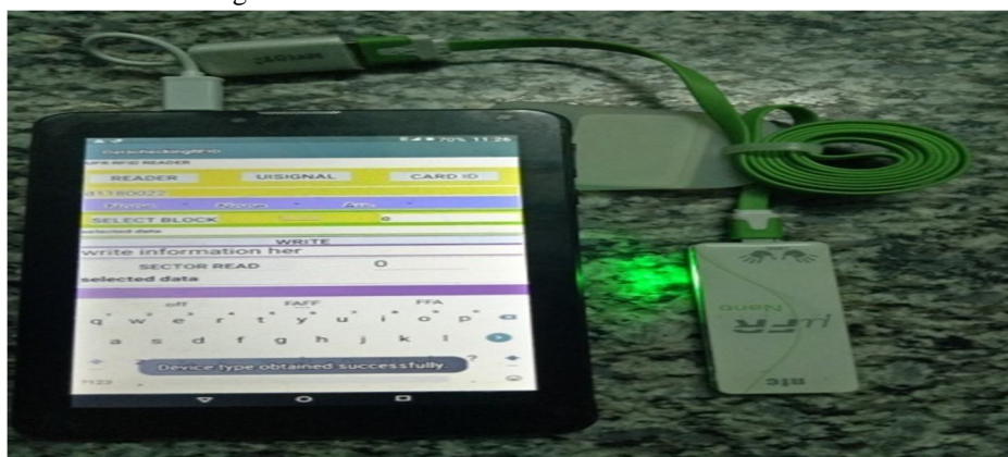
Fig. 4 RFID Based Library self management system using RFID (R/W) with Tab
