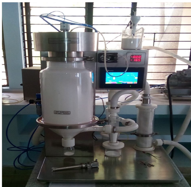
Fig. 2.1. Spray Drying of as-synthesised calcined lanthanum zirconate powder. (Property of CSIR-NAL Bangalore)
