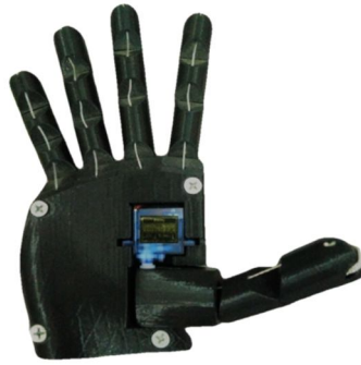
Fig. 2 A Prototype of Robot's Right Arm with Fingers.
