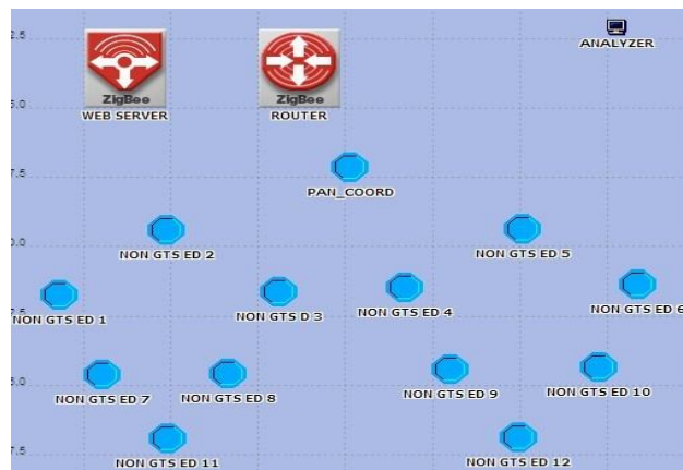
Fig. 3. Variant of 802.15.4 – Without GTS
