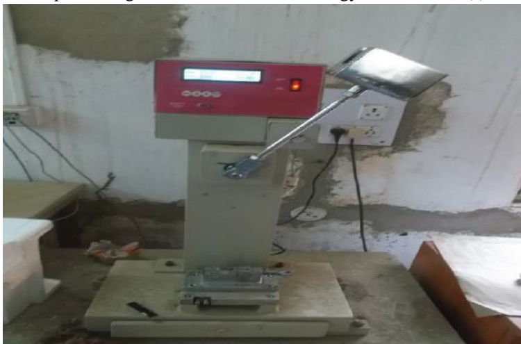
Fig- 3. Experimental set up for Impact Test Machine
