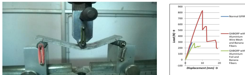
Figure.1 Flexural testing of the specimen (ASTM D 790). Figure 2. Load vs. displacement graphs for flexural test (ASTM D 790)
