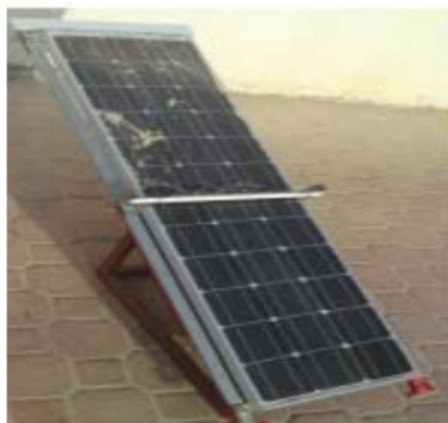
Fig5-b Solar panels with wiper connected
