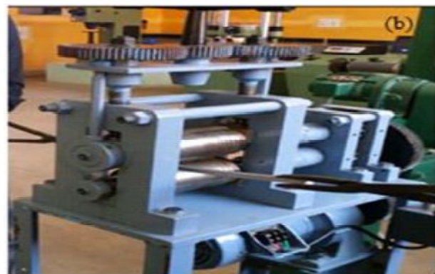
(b) Rolling of composite in a rolling mill
