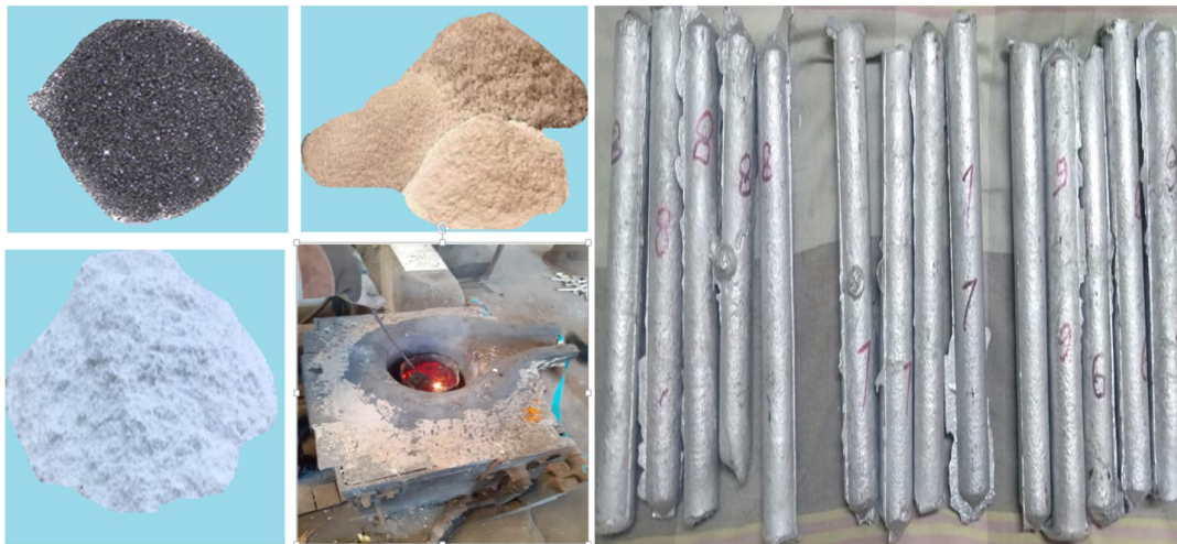
Fig 1.1 stir casting setup and fabricated samples
