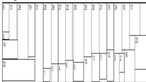
Fig. 5. Physical placement of AMI33, Unused area = 6.888%.
