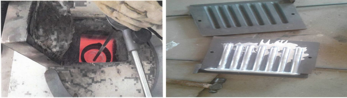
Fig. 1(a) Setup for Casting (b) Fabrication of Fingers in Grey Cast Iron Die
