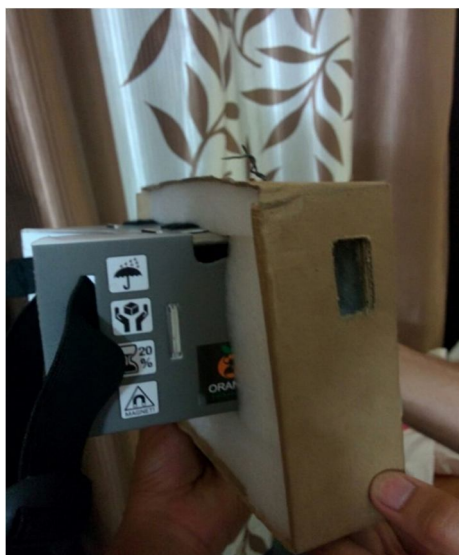
Figure 4.3: Enclosing the VR cardboard and LCD screen in a single box
