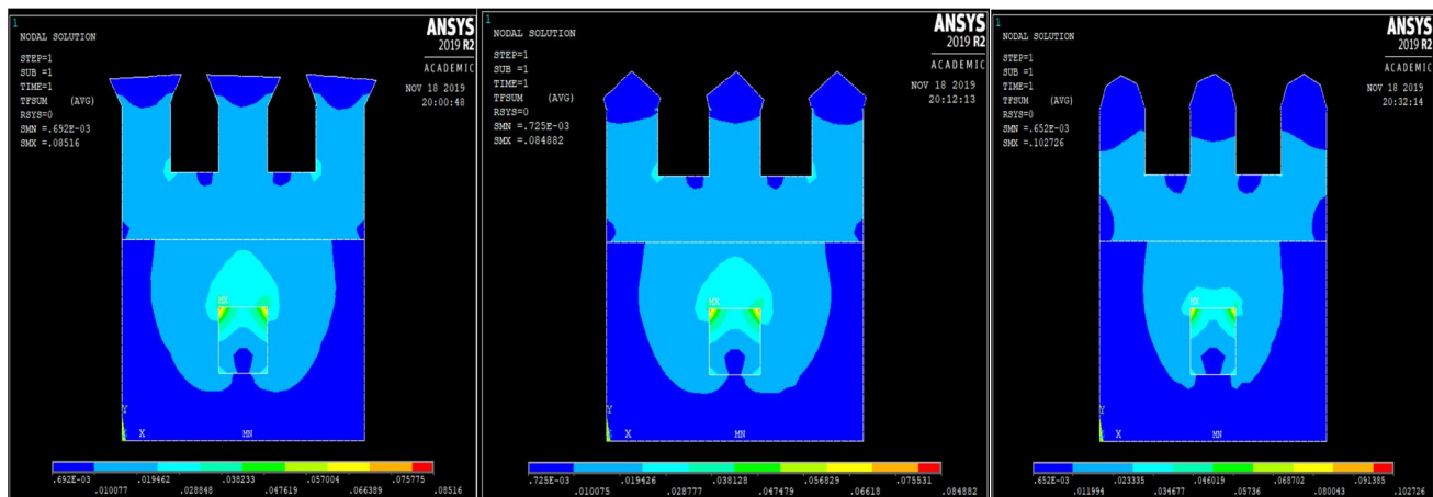
Fig 1.8 Heat Flux of the Triangular, Pentagon & Octagonal I fin model silicon heat source thermal system
