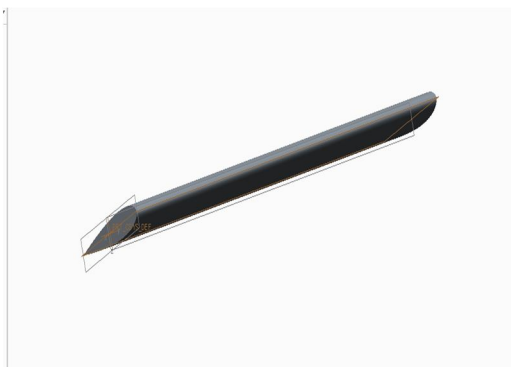
Fig A: 3D model of NACA Aerofoil 0012
