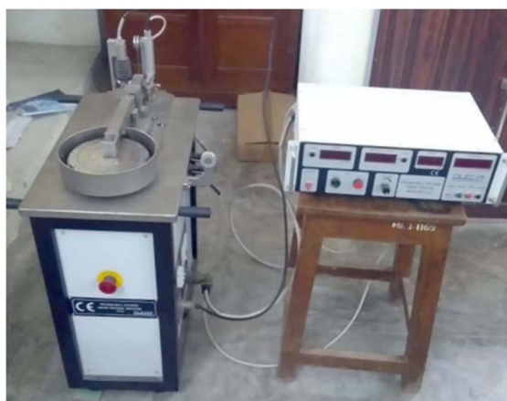
2.2 Pin on Disc wear testing
