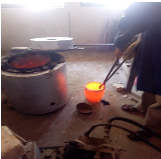
Fig. III Crucible after heating with molten cast iron
