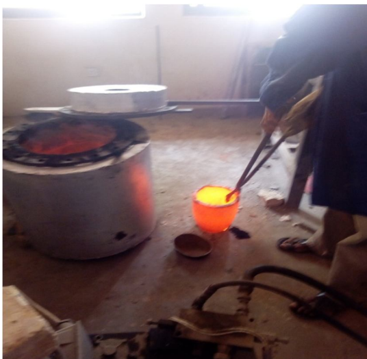
Fig. III Crucible after heating with molten cast iron
