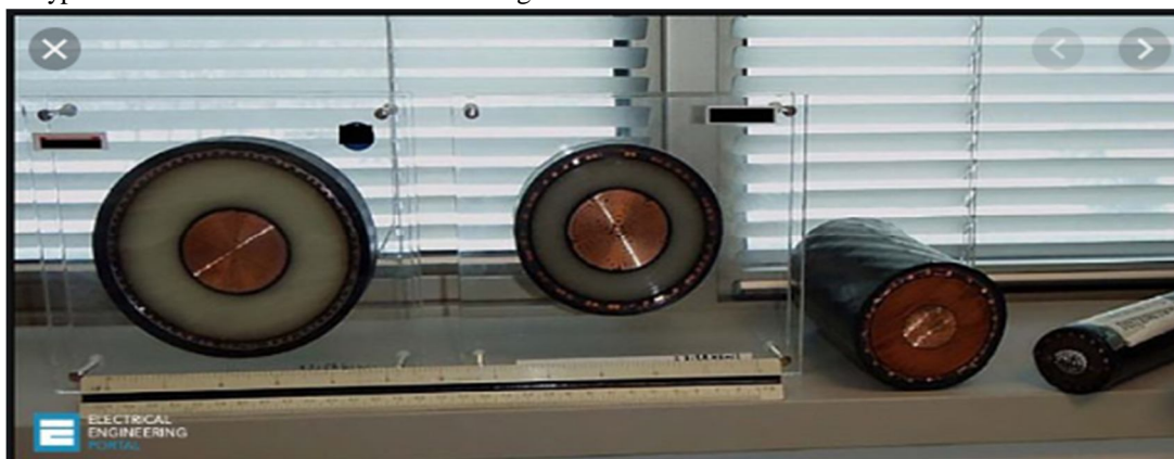
Fig 2: Underground XLPE Cables with Different Ratings
