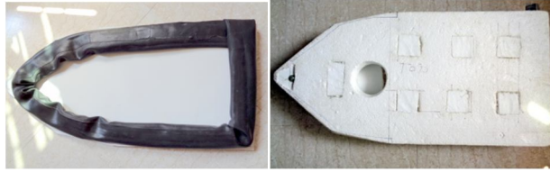
Fig 3.6 This piece is pasted on the depron base by making some hole on the depron and it is fixed with screws
