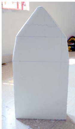
Fig 3.1 Making the base of hovercraft from the material depron sheet
