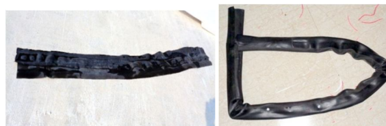
Fig 3.4 A tube like structure is made from two piece of synthetic rubber sheet and it is inserted through the multi-wood strip.
