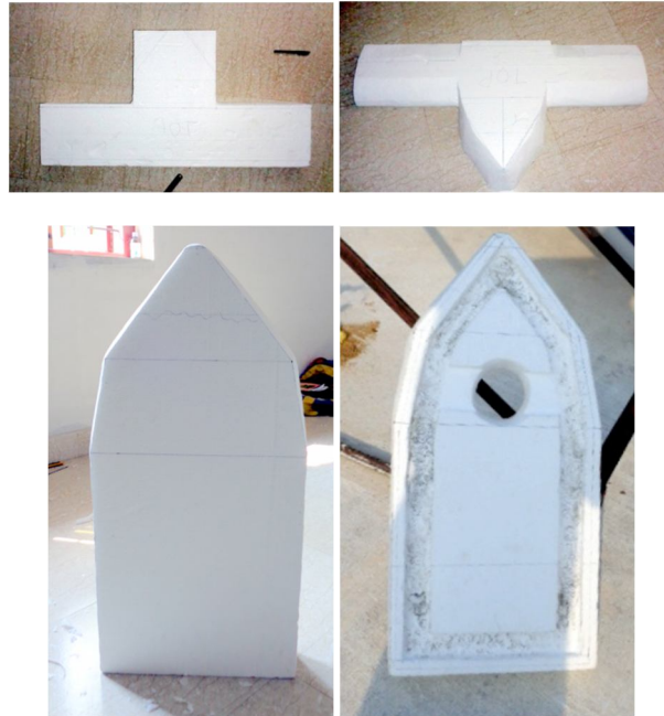
Fig 3.2 A hole of 14cm diameter on the base and a path for the air flow is made
