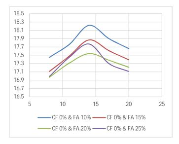
3) Variation of OMC and MDD on addition of coir fiber and fly ash
