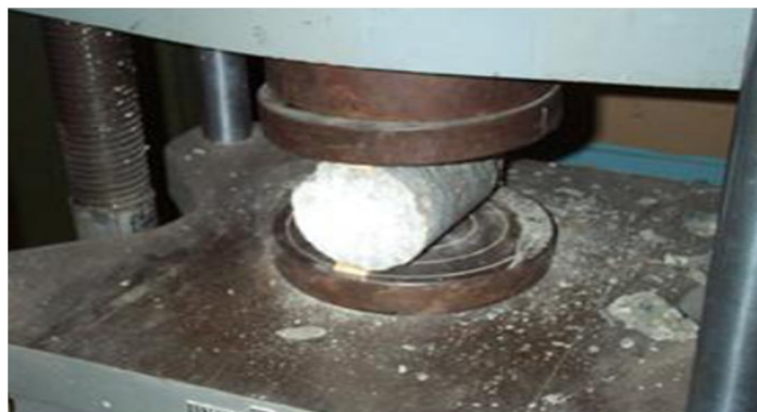
Fig 4.2: Split Tensile Strength Test
