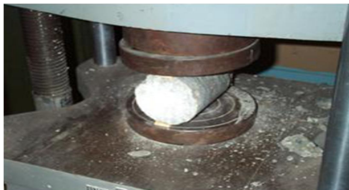
Fig 4.2: Split Tensile Strength Test
