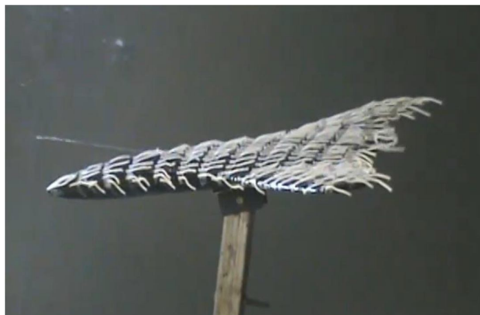
Fig 20: Negative 10 degree angle of attack
