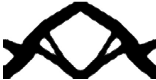
Fig. 5 Shape obtained by Method of Moving Asymptote
