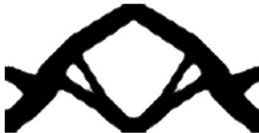
Fig. 5 Shape obtained by Method of Moving Asymptote
