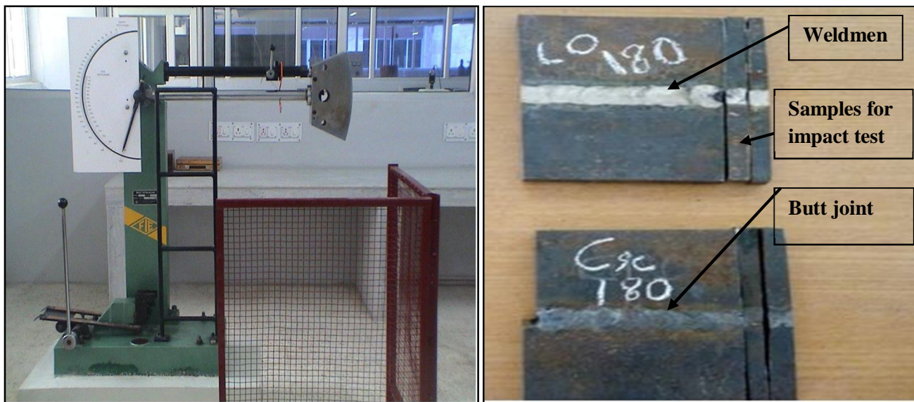
Fig. 2: (a) Impact testing machine (b) Samples for Impact test
