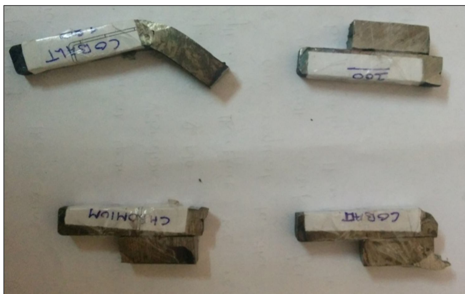
Fig. 3: Impact test samples after test
