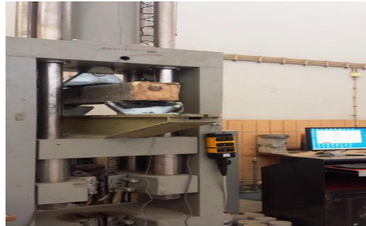
Figure 3 Test Setup of RC beam specimen
