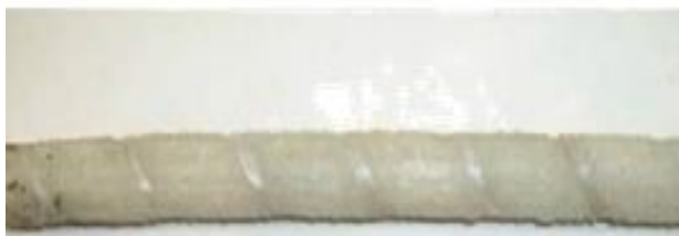
Figure 1 Wrapped Surface GFRP rod with Vinyl-ester resins
