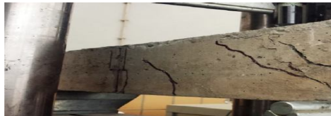
Figure 9 Failure and cracking pattern of specimen
