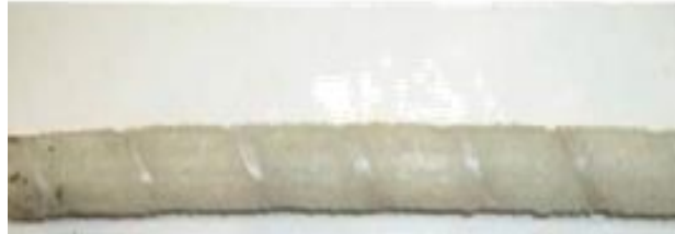
Figure 1 Wrapped Surface GFRP rod with Vinyl-ester resins
