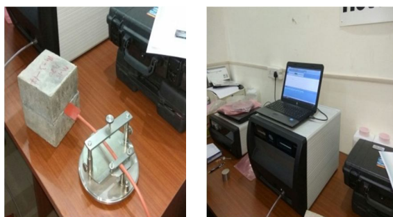
Fig.6: Placing of sensor between two halves of sample and recording of measurements
