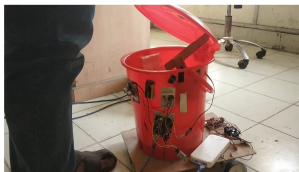
Fig. 15 Trash bin lid open on sensing the user
