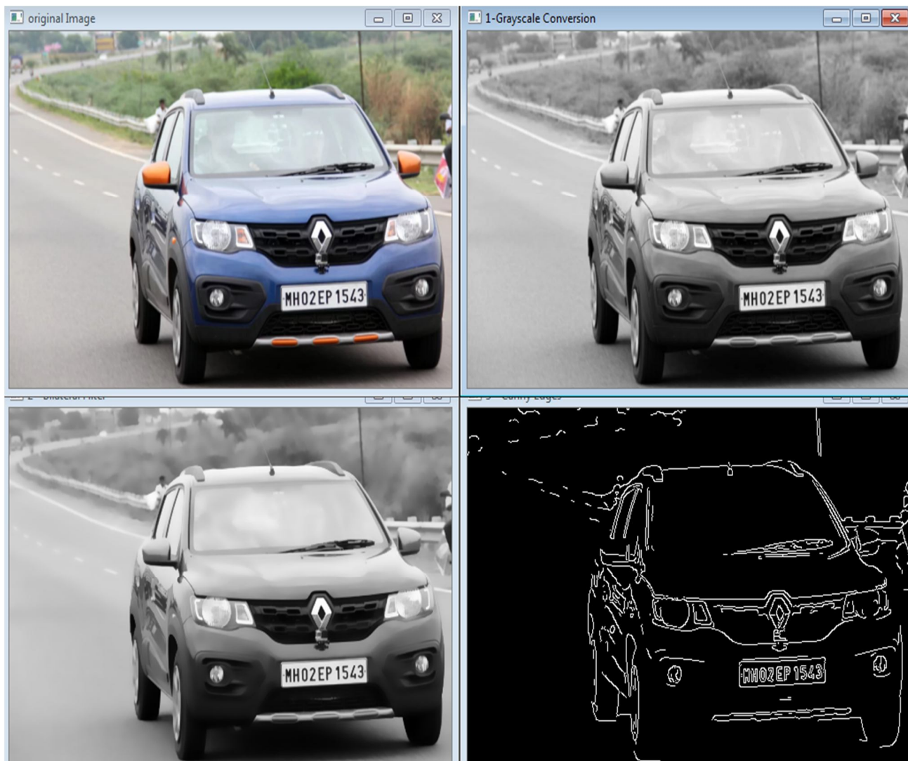
Figure 2: Automatic Number Plate Recognition system acquiring the number plate
