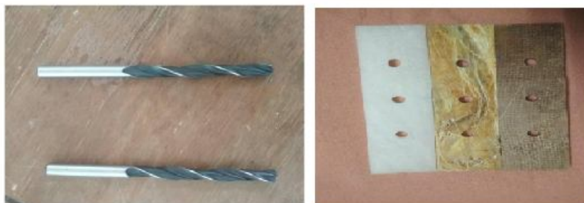
Fig.2.2.4 drill bits Fig.2.2.5Specimens after drilling
