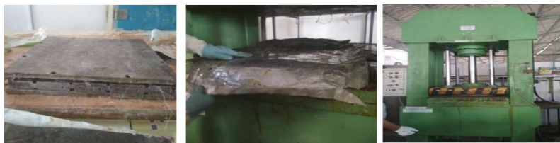
Fig.2.2.2 Placing the enclosed mould in hydraulic press
