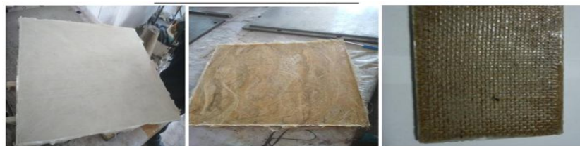
Fig.2.2.3 cotton ,sisal jute natural fiber composite
