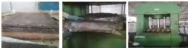
Fig.2.2.2 Placing the enclosed mould in hydraulic press
