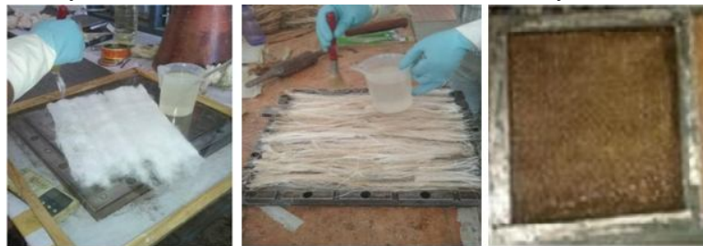
(a) (b) (c) Fig.2.2.1 Preparation of cotton ,sisal ,jute laminate
