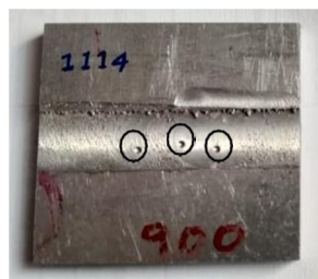
Fig.1.14 900rpm Rockwell Hardness
