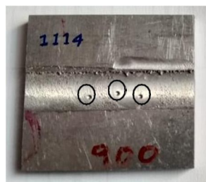
Fig.1.14 900rpm Rockwell Hardness
