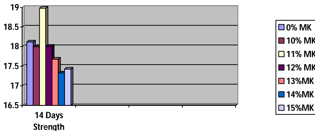
Fig : 18 Graphical representation of 14 Days Compressive strength with different % replacement of MK
