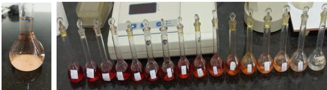
Fig. 12 Standard Flask with varied FAS concentration, 4cm 3 KCNS, and 1.5 HNO 3 cm 3 , filled with distilled water up to flask mark (left side) and different concentration of Ferric solution in Standard flask
