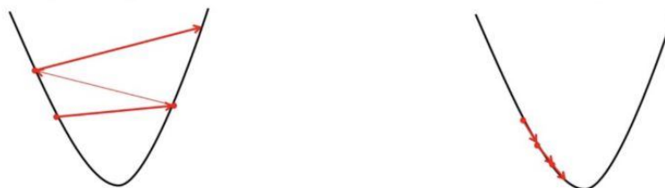
Fig. 11 Learning rate L value is optimized as if too large (left side) gradient Descent can overshoot the minimum and if L is too small Gradient Descent will take small steps to reach local minima and will take a longer time to reach minima.
