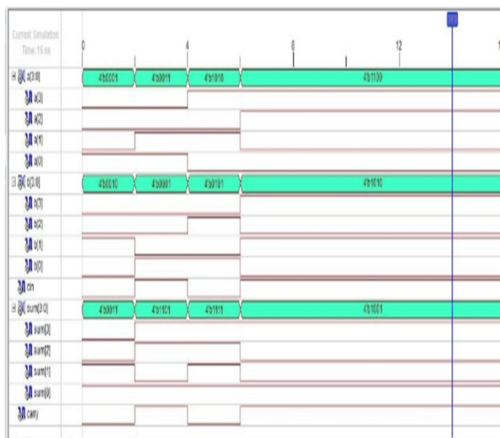
Fig 6 Output waveform of Carry Skip Adder
