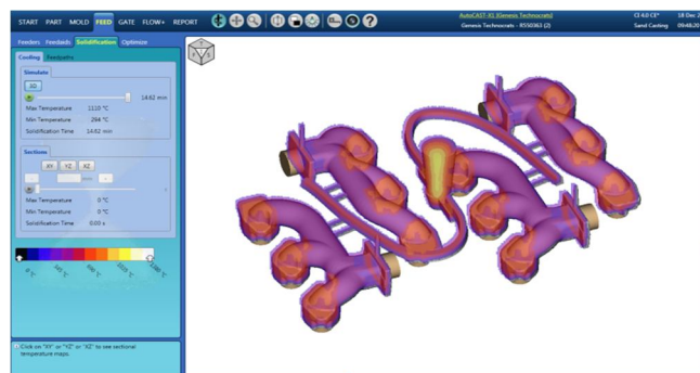
Fig no. 8 Solidification result of modified designed gating
