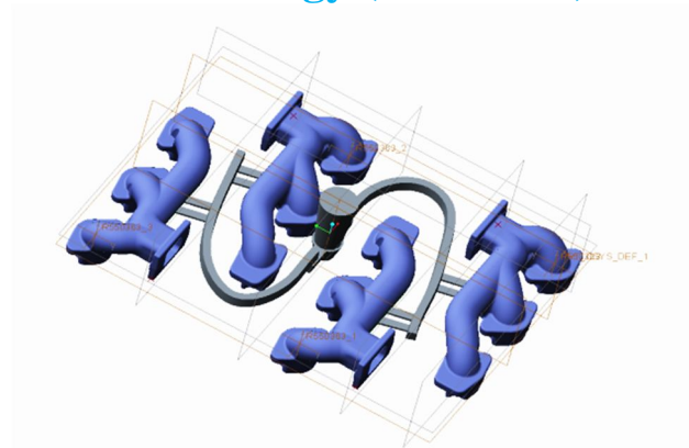
Fig. 4 3D CAD model of casting assembly with old gating design
