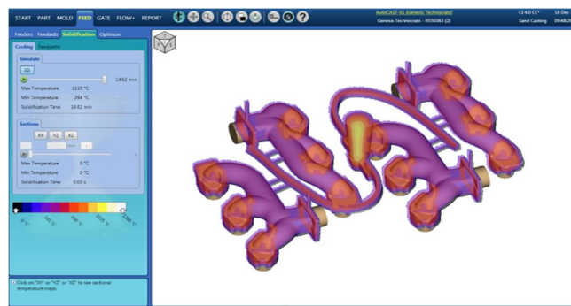
Fig no. 8 Solidification result of modified designed gating
