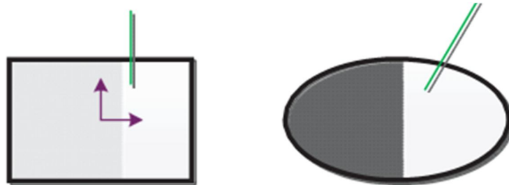
Fig. 5 The tool path of radial drilling.
